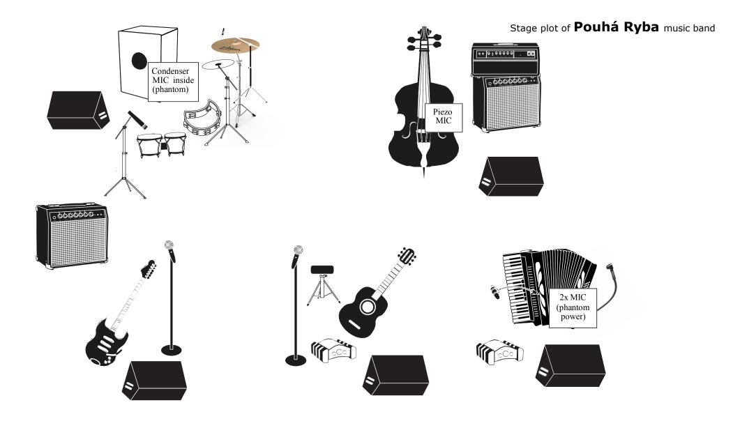
Imput list: <u>Two lead vocal</u> (2mics dymanic), <u>El. guitar</u> (combo line\mic), <u>Acustic guitar</u> (jack- DI box), <u>Double bass\Kontrabas</u> (*phantom* piezo mic, xlr line from combo), <u>Accordion</u> (*phantom* 2mics – DI), <u>Percussion</u> (Cajon-*phantom* kick drum mic, Bongos- instr. mic, Cymbals and Tambourine- condenser mic optional)
